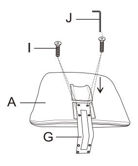
STEP 4: Install the backrest together with seat by fix the metal plate on the seat. Screw: M6x25mm (4pcs) Installation tip: Install the front two screws of the Backrod throught the two screw holes in the tray/mechanism;
